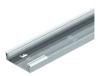
On-floor trunking base, 1 compartment, for blank/mounting lid with slope on one side, with plug-fit aluminium side profiles for layering and fixing the trunking lid, metal floor base with holding shackles for max. two plug-in, self-contacting dividers and groove for earth conductor clamp. Trunking height suitable for installation of Telitanks.
