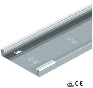
On-floor trunking base, 1 compartment, for blank/mounting lid with slope on one side, with plug-fit aluminium side profiles for layering and fixing the trunking lid, metal floor base with holding shackles for max. two plug-in, self-contacting dividers and groove for earth conductor clamp. Trunking height suitable for installation of Telitanks or service outlets of nominal size 4, 6, 9.
