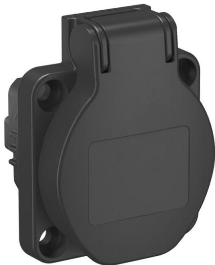
Protective contact extension socket 0° with hinged cover, with screwless terminals, 2-pin, 16 A, 250 V~, with connection terminals to IEC 60884-1. Protection rating: IP44.
