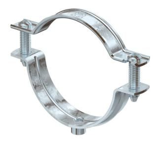
Spacer clip for the installation of pipes and cables on walls, ceiling and floors. With self-locking upper part. Surfaces G and FT from a clip size of 20 are suitable for installation with a nail device or a bolt-firing tool.
