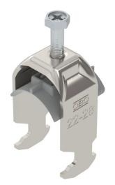
Clamp clip with hammerhead foot, plastic pressure sleeve made of polypropylene. For vertical and horizontal mounting of 1 single cable on a C-profile rail. For a slot width 16–17 mm. With 1-start screw thread on pressure sleeve, universal hexagonal screw head WAF10, with slot and cross recess. Suitable for assembly indoors and outdoors. We recommend the use of a counter-sleeve.
