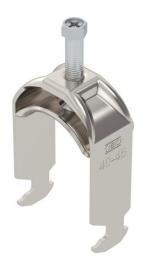
Clamp clip with hammerhead foot, metal pressure sleeve with rounded edges to protect the cable. For vertical and horizontal mounting of 1 single cable on a C-profile rail. For a slot width 16–17 mm. With 1-start screw thread on pressure sleeve, universal hexagonal screw head WAF10, with slot and cross recess. Suitable for assembly indoors and outdoors. We recommend the use of a countersleeve.
