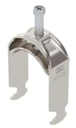
Clamp clip with hammerhead foot, metal pressure sleeve with rounded edges to protect the cable. For vertical and horizontal mounting of 1 single cable on a C-profile rail. For a slot width 16–17 mm. With 1-start screw thread on pressure sleeve, universal hexagonal screw head WAF10, with slot and cross recess. Suitable for assembly indoors and outdoors. We recommend the use of a countersleeve.
