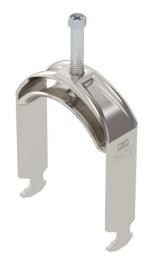
Clamp clip with hammerhead foot, metal pressure sleeve with rounded edges to protect the cable. For vertical and horizontal mounting of 1 single cable on a C-profile rail. For a slot width 16–17 mm. With 1-start screw thread on pressure sleeve, universal hexagonal screw head WAF10, with slot and cross recess. Suitable for assembly indoors and outdoors. We recommend the use of a countersleeve.
