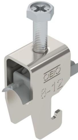
Clamp clip with U-foot, plastic pressure sleeve made of polypropylene. For vertical and horizontal mounting of 1 single cable on a C-profile rail. For slot width 18–22 mm. With 1-start screw thread on pressure sleeve, universal hexagonal screw head WAF10, with slot and cross recess. Suitable for assembly indoors and outdoors. We recommend the use of a counter-sleeve.
