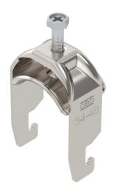
Clamp clip with U-foot, metal pressure sleeve with rounded edges to protect the cable. For vertical and horizontal mounting of 1 single cable on a C-profile rail. For slot width 18–22 mm. With 1-start screw thread on pressure sleeve, universal hexagonal screw head WAF10, with slot and cross recess. Suitable for assembly indoors and outdoors. We recommend the use of a counter-sleeve.
