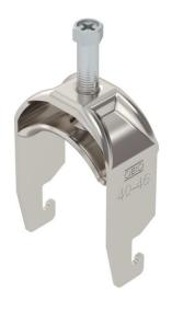
Clamp clip with U-foot, metal pressure sleeve with rounded edges to protect the cable. For vertical and horizontal mounting of 1 single cable on a C-profile rail. For slot width 18–22 mm. With 1-start screw thread on pressure sleeve, universal hexagonal screw head WAF10, with slot and cross recess. Suitable for assembly indoors and outdoors. We recommend the use of a counter-sleeve.
