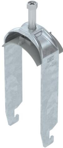
Clamp clip with U-foot, plastic pressure sleeve made of polypropylene. For vertical and horizontal mounting of 2 single cables on a C-profile rail. For slot width 18–22 mm. With 1-start screw thread on pressure sleeve, universal hexagonal screw head WAF10, with slot and cross recess. Suitable for assembly indoors and outdoors. Multiple cables should be separated by double sleeves. We recommend the use of a counter-sleeve.
