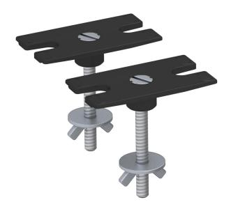
Fastening set for fixed mounting of a Deskbox, type DB, under the tabletop. It is mounted using a drill hole (Ø10 mm) in the tabletop.
