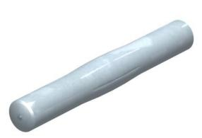
Joint connectors as notched pins for direct joint-to-joint connection of the trunking bases without joint cover. Suitable for aluminium device installation trunking of the Rapid 80 and Rapid 45-2 series and GAD design trunking for system use for cable routing and/or with Modul45 connect. Also compatible with the BK 1874 floor trunking.
