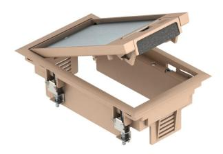
Service outlet with handle clamp for up to 3 individual Modul 45 devices in one UT3 universal support, use in duct systems and system floors for indoor use. Up to two installation devices with 50 mm central plate can be inserted. Service outlet with handle clamp, 1-compartment, for the installation of MT2 mounting support.
