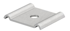
Hold-down clamp for fastening mesh cable trays. Including lens head screw. Use on mesh cable trays with 50 x 100 mm grid only.
