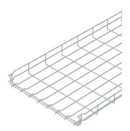
Mesh cable tray with shaped connector of side height 55 mm. No additional connection components are required for the mesh cable tray, it is simply interlocked. The grid width is 50 x 100 mm (exception: GRM 55/50 = 20 x  $^{\circ}$
