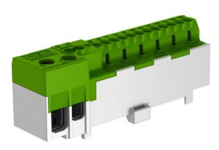
Neutral conductor connection terminal with 12 plug-in terminals,  $2.5 \text{ mm}^2$  or  $1.5 \text{ mm}^2$ , flexible with wire end sleeve; two plug-in terminals,  $4 \text{ mm}^2$  and  $2.5 \text{ mm}^2$ , flexible with wire end sleeve and two screw connection terminals up to  $25 \text{ mm}^2$  or  $16 \text{ mm}^2$ , flexible, 3 Nm. For snapping onto 15 mm hat rails according to DIN EN 60715 (formerly DIN EN 50022).
