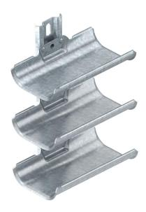
Cable support brackets for quick and easy routing of cables in areas where common cable support systems cannot be installed due to lack of space. The cable support brackets possess a large load-bearing surface as well as rounded outer edges to protect the cables.
