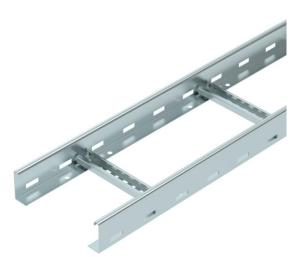
Cable ladder with a 60 mm side height with welded C30 profile rungs which are open in an upwards direction. Rolled side rail for reinforcement and as edge protection. Fastening to the bracket takes place using hold-down clamps, type LKS 40. The slot dimension of the rung is 16.5 mm and the appropriate clamp clip is type BS-H....
