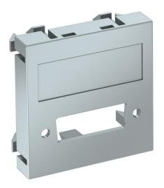
Multimedia support for a DVI plug connector, straight cable outlet, with labelling panel, without plug connector. Support plate with locking fastening, suitable for horizontal and vertical installation in the system environment.
