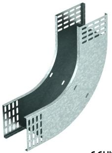
90° rising vertical bend, for all cable tray types of 110 mm side height. The vertical bend is pushed over the end of the cable tray and screwed tight. Fastening materials should be ordered separately.
