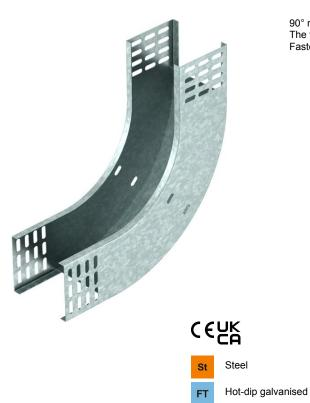
90° rising vertical bend, for all cable tray types of 85 mm side height. The vertical bend is pushed over the end of the cable tray and screwed tight. Fastening materials should be ordered separately.
