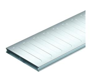
Underfloor duct (2 piece) for routing cables in screed-covered underfloor systems, according to EN 50085-2-2. Removable and continuously lockable trunking cover. With separating retainers in the trunking base. Maximum load-bearing capacity to  $1.5\ kN$ .
