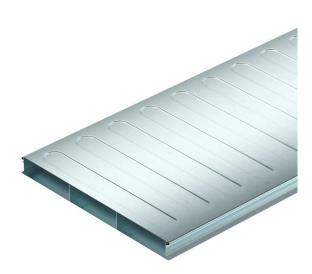
Underfloor trunking (2 piece) for routing cables in screed-covered underfloor systems, according to EN 50085-2-2. Removable and continuously lockable trunking cover. With separating retainers in the trunking base. Maximum load-bearing capacity to 1.5 kN.
