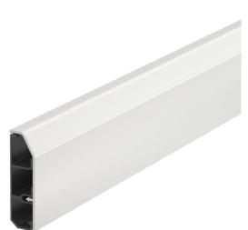
SL skirting trunking for covered cable routing in internal areas. The colour of the trunking bases can vary depending on the production method. With snap-on cover and base, with base perforation for direct wall mounting. Change the direction with the fittings and close the trunking ends with end pieces. Service outlet for installing power and data technology. Tested according to DIN EN 50085-1 and DIN EN 50085-2-1.
