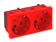
Protective contact socket Double 33°, encoded version, with increased touch protection, with screwless terminals, 2-pin, 16 A, 250 V $\sim$ , with connection terminals according to IEC 60884-1.
