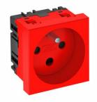
Socket with earthing pin, single  $0^\circ$ , encoded version, with increased touch protection, with screwless terminals, 2-pin, 16 A, 250 V $\sim$ , with connection terminals according to IEC 60884-1.
