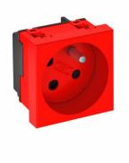
Socket with earthing pin Single 33°, encoded version, with increased touch protection, with screwless terminals, 2-pin, 16 A, 250 V $\sim$ , with connection terminals to IEC 60884-1. The socket can only be used in conjunction with an encoding pin, type CST-STD.
