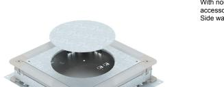
Underfloor accessory box for screed-covered underfloor installation ducts with sheet steel side walls. To mount installation units of the selected nominal size. Height can be infinitely adjusted to the nominal screed height (rapid adjustment possible) and the screed can be worked flushed to the screed scraping edge. With noise decoupling option after screed laying and can be used with system accessories, also for heavy-duty application.
