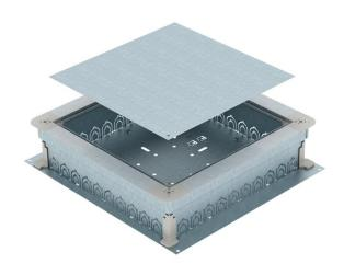
Underfloor junction and branch box for 10 installation pipes on each side (M20 or M32) with sheet steel side walls. To mount installation units in the mounting lid (to be ordered separately). Height can be infinitely adjusted to the nominal screed height (rapid adjustment possible) and the screed can be worked flushed to the screed scraping edge. With noise decoupling option after screed laying and can be used with system accessories, also for heavy-duty application.
