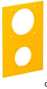
Cover plate with a Ø 45 mm opening for the installation of one extension socket (type ASD-...) with 38 mm fastening track and a Ø 60 mm opening for the installation of one CEE socket 16/32 A with 60 mm fastening track, including 8 screws for fastening the device.
