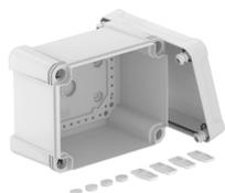
Junction box for the connection of cables and lines indoors and in outdoor areas. Rectangular design without entries. Suitable for wall and ceiling mounting with the option to fasten outside, inside or to mount via the corner domes. Particularly impact resistant with IK09. Cover with quick lock, sealable. Made from halogen-free and UV-resistant materials.
