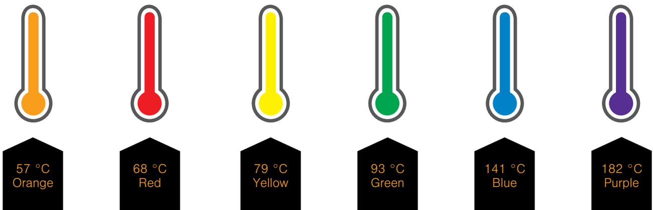
Different trigger temperatures of glass vials on the sprinkler head
