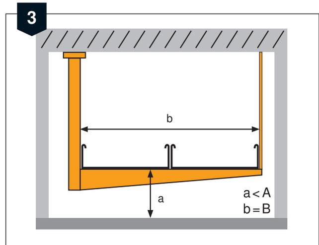
The basic data was determined in the fire tests. This data allows the design of various variants if, for example, there is no mounting space available at the side or if deformation should be restricted further.
