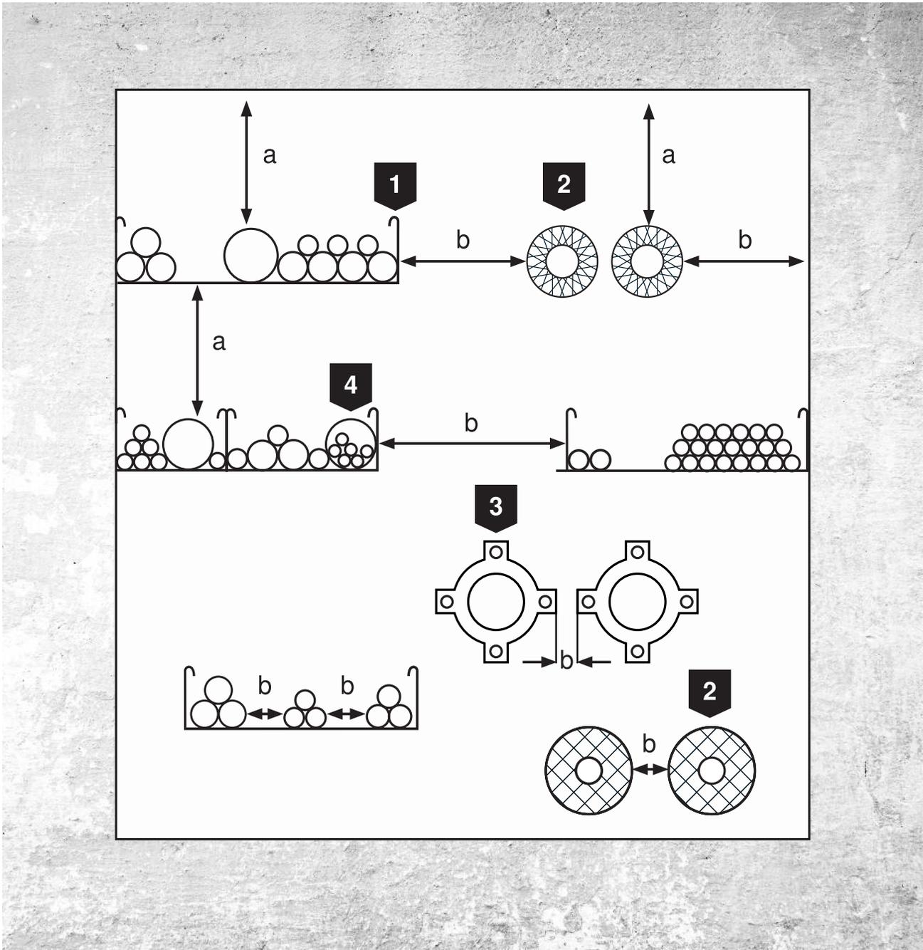
Spacings between the installations and to the component
