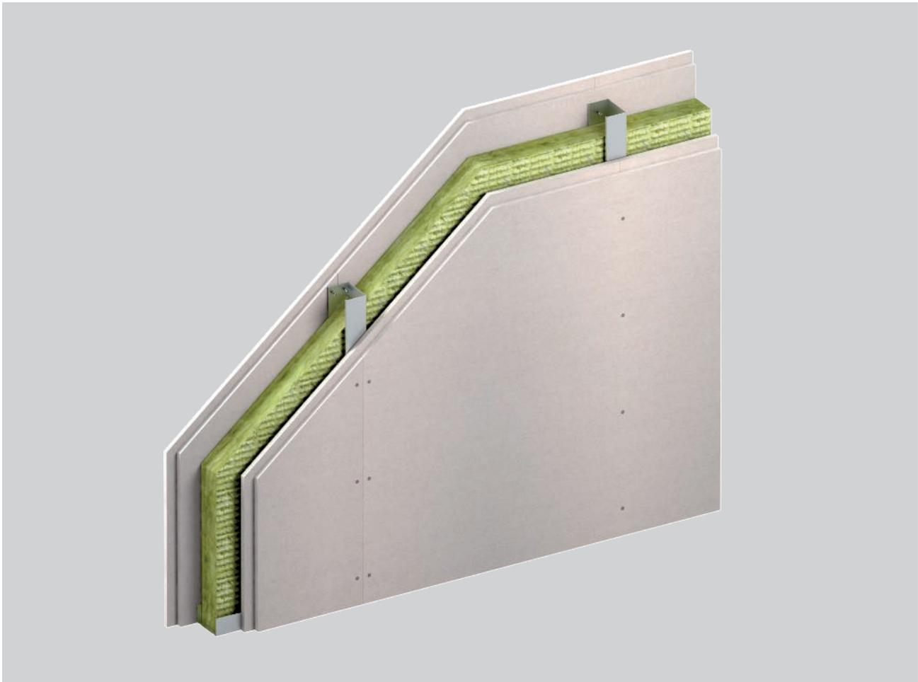
*Partition construction with plasterboard plates*
