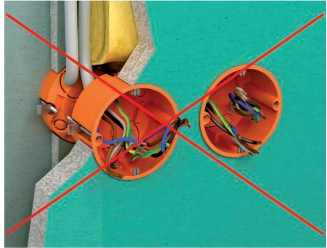
Unapproved installation of opposing standard cavity wall sockets in lightweight partitions with fire resistance.
