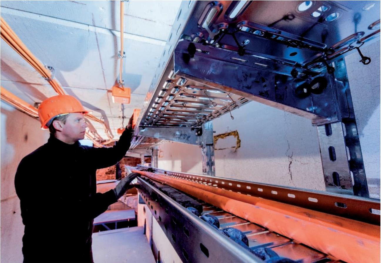
Test structure of a cable system that maintains electrical functionality
